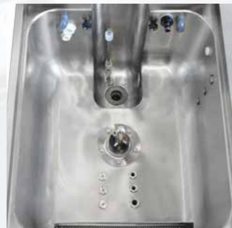
Some areas around the **washing tank** have the purpose to gather all dirty materials and to guarantee the proper working of the washing cycle's phases. A frontal filtered zone catches the superficial dirt; a second backward zone guarantees the correct filling levels' functioning. A lower little tank collects finally the dirty that's on the tank bottom.
